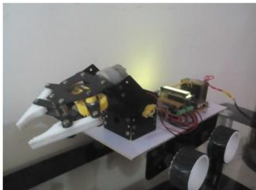
Fig: 4.2 Figure indicate the robot jaw is open.
